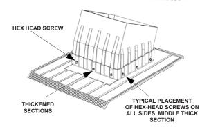
14. Run a bead of clear silicon along the inside of the joins if necessary.
