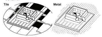
7. From inside the roof space ensure the orientation of the dropper base is correct. Clip the dropper base onto the underside of the flashing. Ensure there are no obstructions to the flexible duct adaptors.
