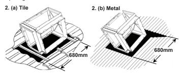
4. Pack the opening with timber off cuts if the distance between trusses is exceeds 550mm
