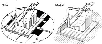
15. If it is desirable to trim the top of the dropper do not trim off more than 100mm. Place the unit on top of the dropper, level and fix in position.
