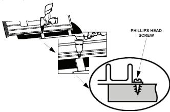
11. Place the required top section on the flashing: Angled top for most common units. Straight top for Breezair contour units
