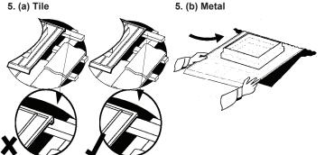
6. Ensure flashing is square with the roof tiles/roof line and using the hexagonal head screws provided, loosely install one screw per side to hold the flashing in place. DO NOT FASTEN THESE TWO SCREWS.
